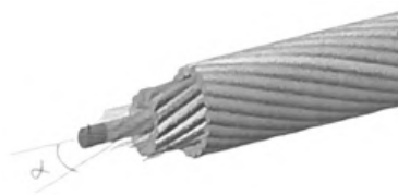
Figure 1.2: Standard composition of the cable.
